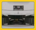
Horizontal Angle Measurement Horizontal angles can be read in 1° or 1gon units. The freely rotatable circle allows any angle reading from zero. Right angles can be quickly set for layout and alignment tasks.
