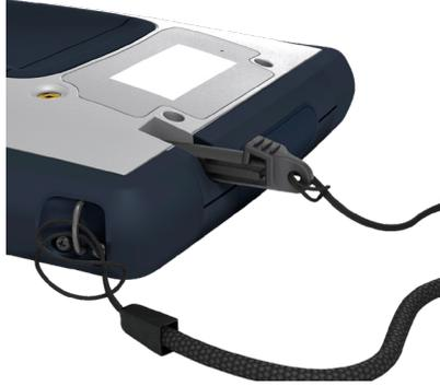
3. Insert the stylus with the attached tether through this loop and tighten the loop.
