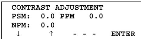
This enables you to adjust the brightness by pressing the [F1](↓) or [F2](↑) key.
