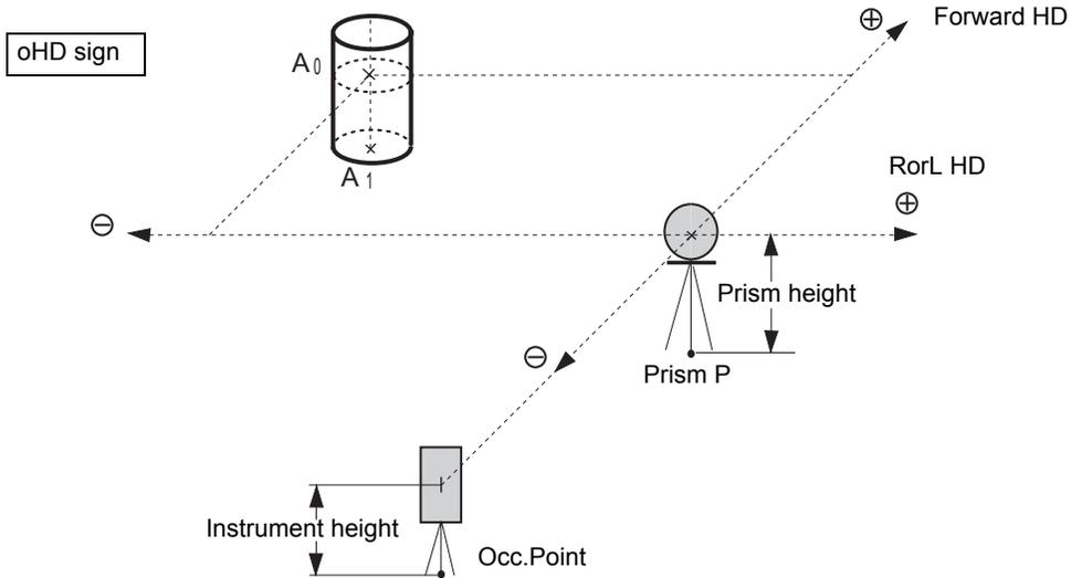
When measuring coordinates of ground point A<sub>1</sub>:
