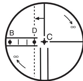
3) Shift the vertical cross-hair line and coincide it with Point D, by revolving the left and right capstan adjustment screws with the adjusting pin. Upon completing the adjustment, repeat the checking operation once more.
