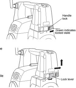
2. Pull the lock levers towards you and slide the handle back and up to remove. The handle lock levers, once released, will return to the original position.
