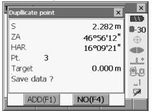
Press **[ADD]** to record the point as another record with the same name. Press **[NO]** to input a new name.
