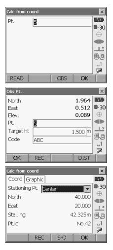
4. Press **[OK]** in the screen shown in step 3 to display the coordinates and point number of the center peg and width peg.
