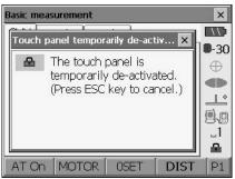
The touch panel cannot be operated while the above message is displayed. Press **{ESC}** to cancel the message and re-activate the touch panel.
