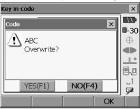
Press **[NO]** to input a new code. Press **[YES]** to overwrite the present code.
