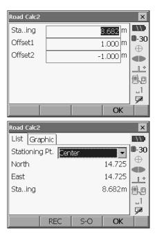
10. Press **[OK]** in the screen shown in step 9 to calculate the coordinates and stationing chainage of the center peg and width peg. The results are then displayed on the screen.
