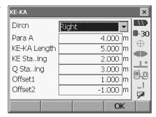
Press [OK] in the screen shown in step 6 to calculate the center peg and width peg coordinates and azimuth angle. The coordinates and azimuth angle are then displayed on the screen.
