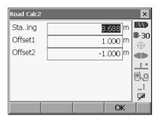
Press [OK] in the screen shown in step 9 to calculate the coordinates and stationing chainage of the center peg and width peg. The results are then displayed on the screen
