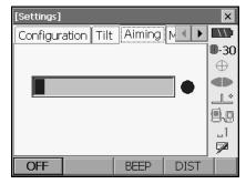
When **[AIM]** is pressed, a gauge indicating light intensity is displayed.
