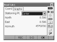
8. Press **{ESC}** repeatedly to finish Clothoid Curve calculation and return to <Road>.
