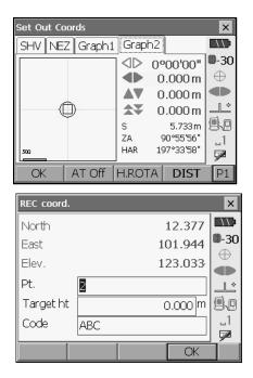
•When recording data in the current JOB, press **[REC]**. Enter point number, target height and code, then press **[OK]**.
