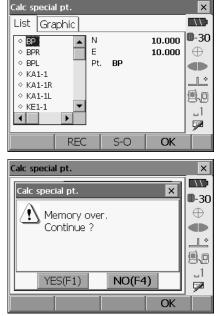
The screen at right is displayed, when the amount of set pegs exceeds 600 points. Press [YES] to continue using the initial 600 points. Press [NO] to return to the screen of step 4.
