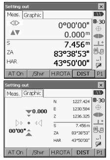
• When recording data in the current JOB, press **[REC]** in page 2. Enter point number, target height and code, then press **[OK]**.
