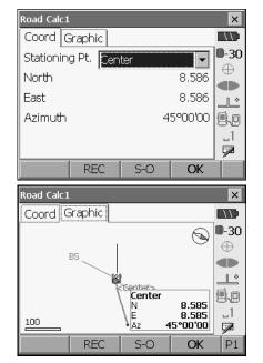
• Select the Graphic tab to display calculation results on a graph.
