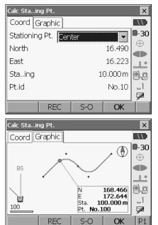
• Select the Graphic tab to display calculation results on a graph.
