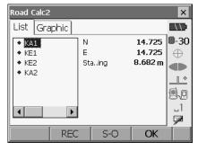
8. Press **[OK]** in the screen shown in step 7 to move to center peg settings.
