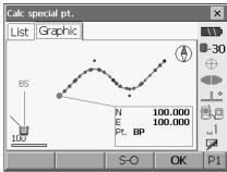
• When "Existing pt." in step 4 has been set to "Skip" a point with a point number which already exists in the current JOB will not be automatically stored. These points are marked with a blue circle. At this stage of the process it is possible to store such a point under a new point number.
