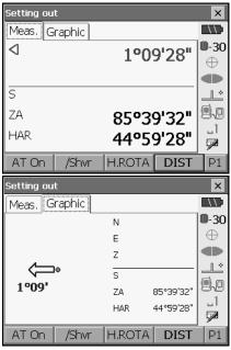
Position the target on the line of sight and press [DIST] to begin distance measurement. The distance and direction to move the target until the setting out point is located is displayed on the SRX. The sighting point measurement results (currently installed position of the target) are displayed.
