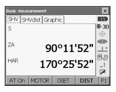
The measured distance data (S), vertical angle (ZA), and horizontal angle (HAR) are displayed.
