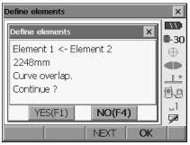
Press **[YES]** to ignore the overlapping and continue calculation. Press **[NO]** to stop calculation and return to the curve properties input screen.
