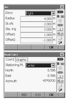
Press [OK] in the screen shown in step 6 to calculate the center peg and width peg coordinates and azimuth angle. The coordinates and azimuth angle are then displayed on the screen.
