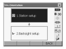
Select "Backsight setup" in <Stn. Orientation> and enter backsight station data.
