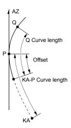
Calculation using KE2 as reference: "KE-KA Calculation"
